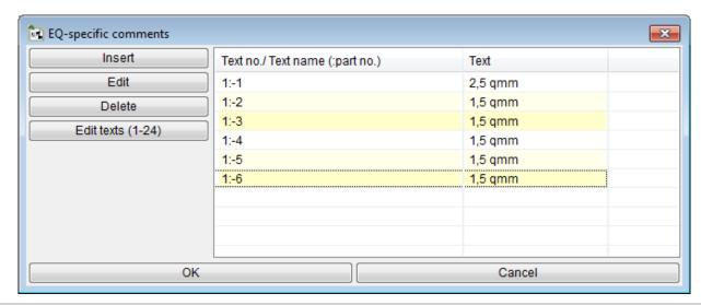
In our example the text "2,5 qmm" was entered in the first connection text of the first connection. For the connection 2 to 6, the text "1,5 qmm" was entered in the first connection text.
