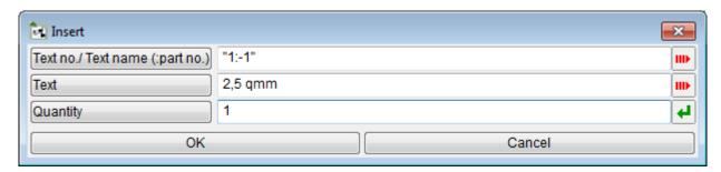
In this screen shot you see, how the text "2,5 qmm" is entered into the 1st connection text of the 1st connection.
